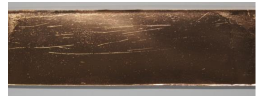
Patterning on PTFE; L/S=50/50μm
