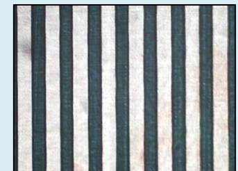
Patterning on PTFE; L/S=50/50μm
